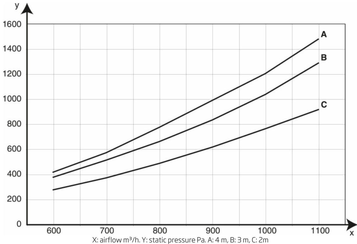
X: airflow m<sup>3</sup>/h. Y: static pressure Pa. A: 4 m, B: 3 m, C: 2m
